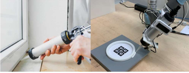
Fig. 1. (Left) Illustration of silicone sealing performed by a human expert and (right) by a robot arm.
