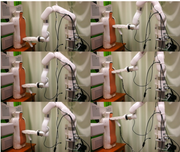
Fig. 7. Force strategy learning at different locations of the phantom's back. Three locations are located at the lumbar region ( left column ) and the other three locations are located at the thoracic region ( right column ).
